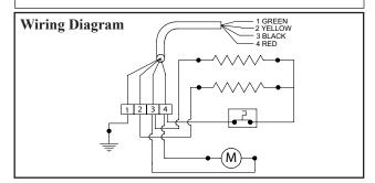
Two wattage configurations are possible: (750W or 1500W).
